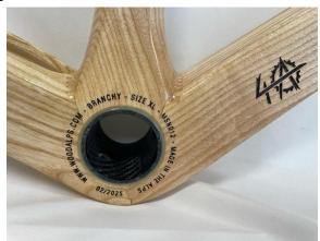
Adapters allow most cranksets, Shimano, Sram, or others, to be installed. Example of an adapter to install a BSA threaded bottom bracket (TOKEN TK4624).
