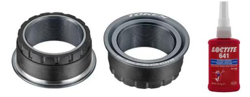
Although there are generally no issues, it is recommended to use LOCTITE 641 adhesive between the adapter and the carbon insert to ensure there are no micro-movements that could generate noise.
