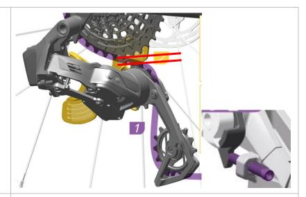
High and low derailleur limit adjustment
