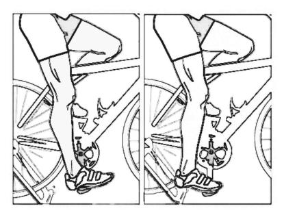
**Fore-Aft Position:** Align knee cap with the pedal axle when pedals are horizontal (use a plumb line for accuracy).
